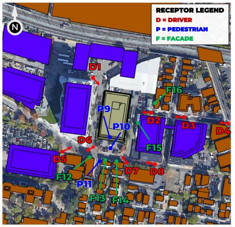
Figure 7: Receptor Locations (Map Underlay Credit: Microsoft Bing Maps) Detailed Solar Reflection Study |
