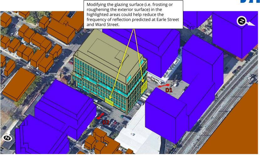
Figure 8: Markup of East and North Facade Locations Where Exterior Surface Modification Could be Considered
