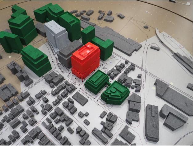
Image 2C: Wind Tunnel Study Model – Full Build Configuration
